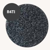
The patented material R4TI is a composite material based on thermoplastic polymers reinforced with carbon fiber. The carbon fiber provides strenght and rigidity. The R4TI can be utilised in any industry but the food and pharmaceutical. Characteristics: Dust free, self-lubrication, high chemical corrosion resistance, temperature range up to 150°, lightness.
