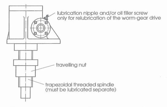
The trapezoidal threaded spindle and worm-gear drive are two separate lubrication points.
