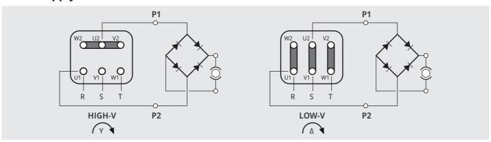
Separate supply: connect directly the supply to the terminals P1 and P2
