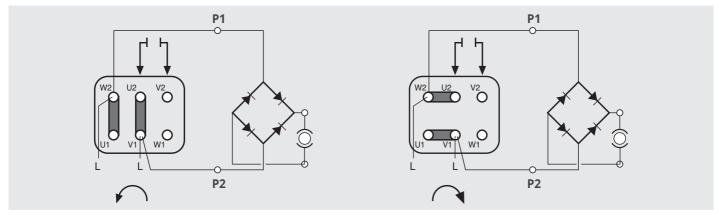
**Separate supply:** connect directly the supply to the terminals P1 and P2.
