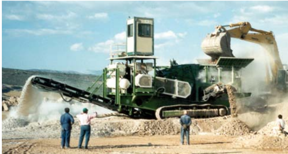
Fig. 10 Planox®-clutch type PMA-HR 183/0 combined with a Voith turbo coupling 650 TG in one of the biggest crusher plants. Engine output P = 550 kW at n = 2100 min -1
