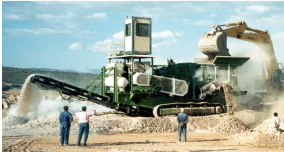
Fig. 10 Planox®-clutch type PMA-HR 183/0 combined with a Voith turbo coupling 650 TG in one of the biggest crusher plants. Engine output P = 550 kW at n = 2100 min -1
